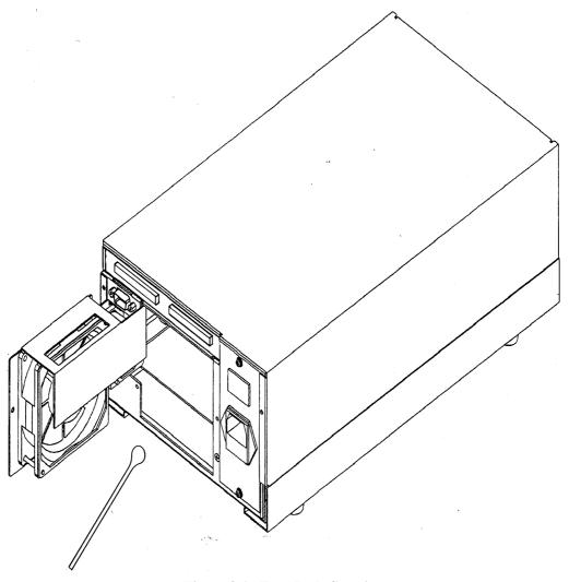
Figure 8-1. Tape Path Cleaning
